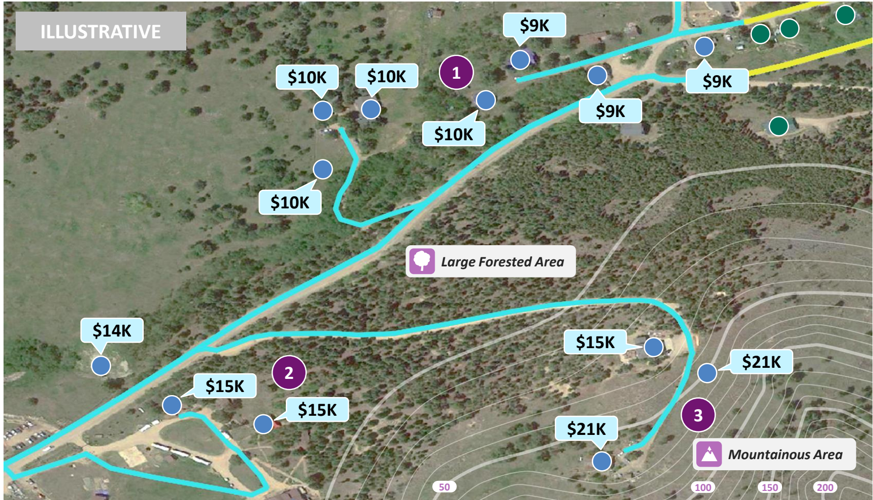
$ Fiber Deployment Cost ● Served Location ● Unserved or Underserved Location — New Fiber Build — Existing Network
